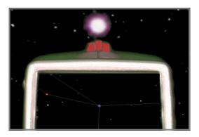
First, line up the light on the front between the two lights on the back. Then line up the object you wish to identify just above the front light. Pull the TRIGGER and mySKY will identify the object you were pointing at.
